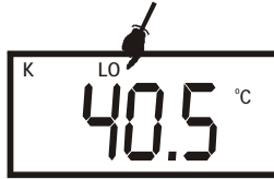
Figure 5: Low battery indicator
