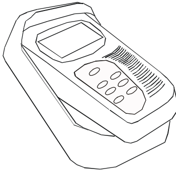
Figure 3: Inserting meter into the rubber boot
