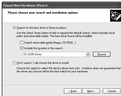
Figure 7 : Select “USB Driver” from the Alpha Link 600 Installation CD
