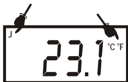
Figure 10: J/K/T and temperature annunciators
