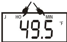
Figure 13: Maximum & minimum HOLD mode
