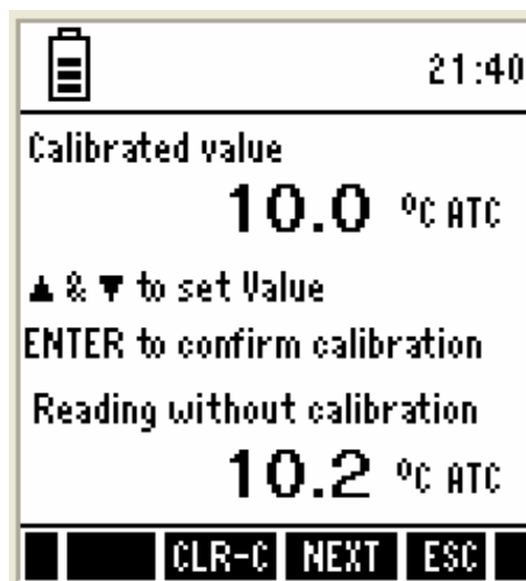
Figure 27: Temperature calibration screen
